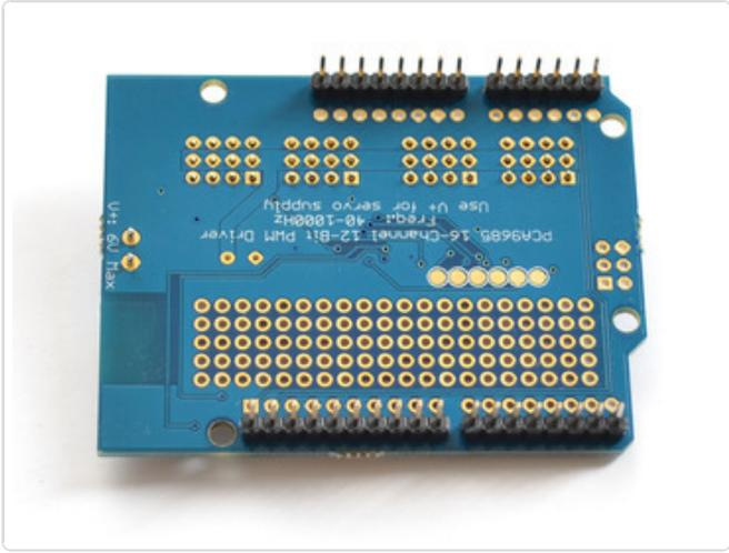
Flip the board over and solder the terminal block
