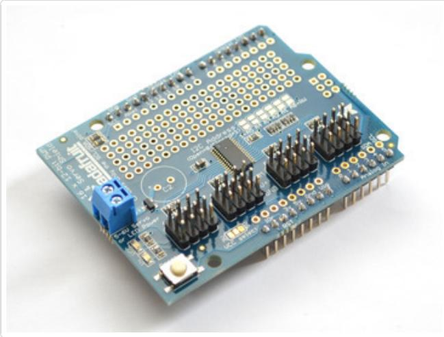
Place the 2 pin terminal block so it faces out. Also place the 3x4 headers so the short pins are plugged into the shield and the long pins are sticking up
