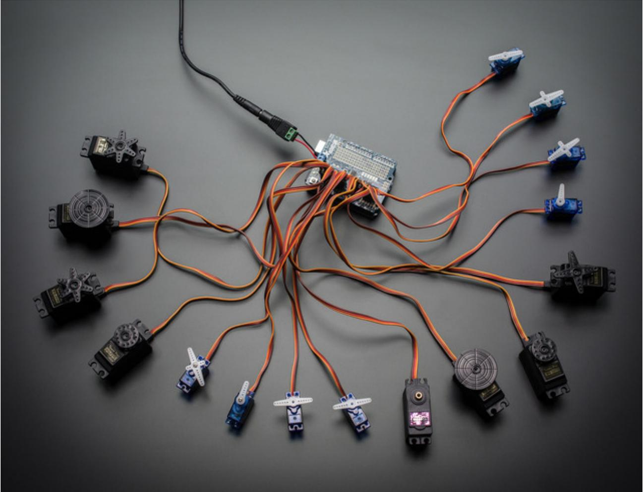
Driving servo motors with the Arduino Servo library is pretty easy, but each one consumes a precious pin - not to mention some Arduino processing power. The Adafruit 16-Channel 12-bit PWM/Servo Driver Shield will drive up to 16 servos over I2C with only 2 pins. The on-board PWM controller will drive all 16 channels simultaneously with no additional Arduino processing overhead. What's more, you can stack up to 62 of them to control up to 992 servos - all with the same 2 pins!
