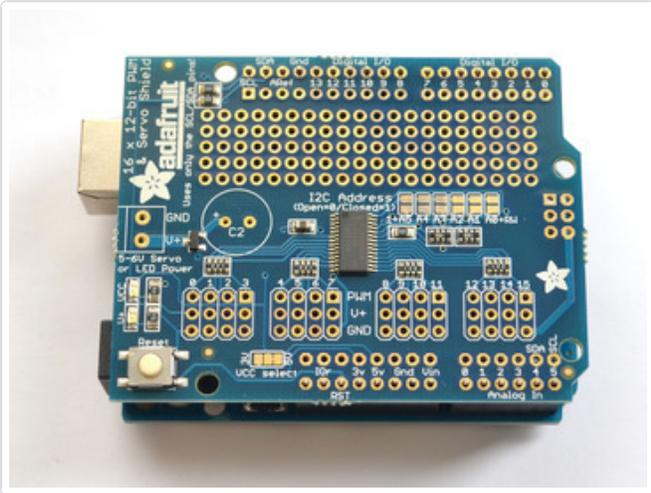
Place the shield on top of the header pins, they should fit into each of the holes along the edge
